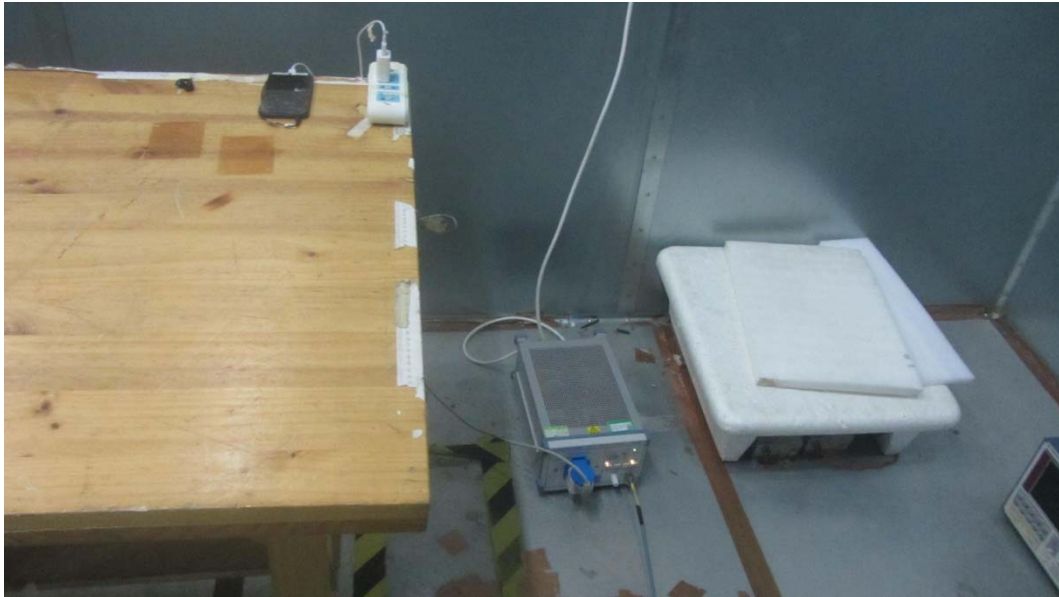
Picture 2 Conducted Emission Test Setup
