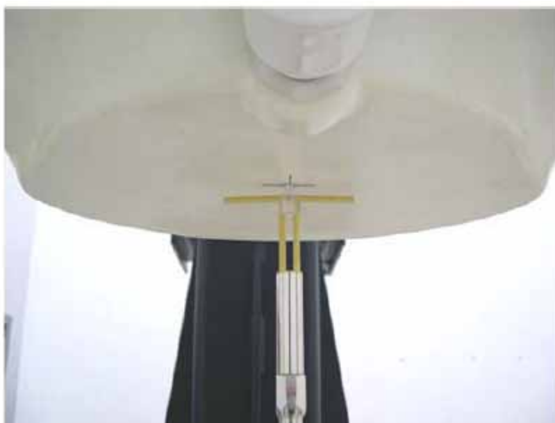
Fig 7.2 Setup Photo of Dipole Antenna
