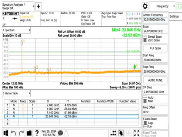
Spurious Emission_BLE 2M_LowCH00-2402MHz
