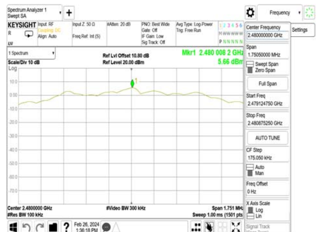
Reference Level_BLE 2M_HighCH39-2480MHz
