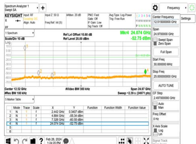
Spurious Emission_BLE 1M_MidCH20-2442MHz
