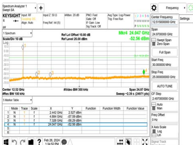
Spurious Emission_BLE 2M_MidCH20-2442MHz
