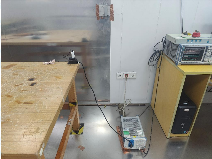
Photo of Setup for Radiated Emission (30MHz~1GHz)
