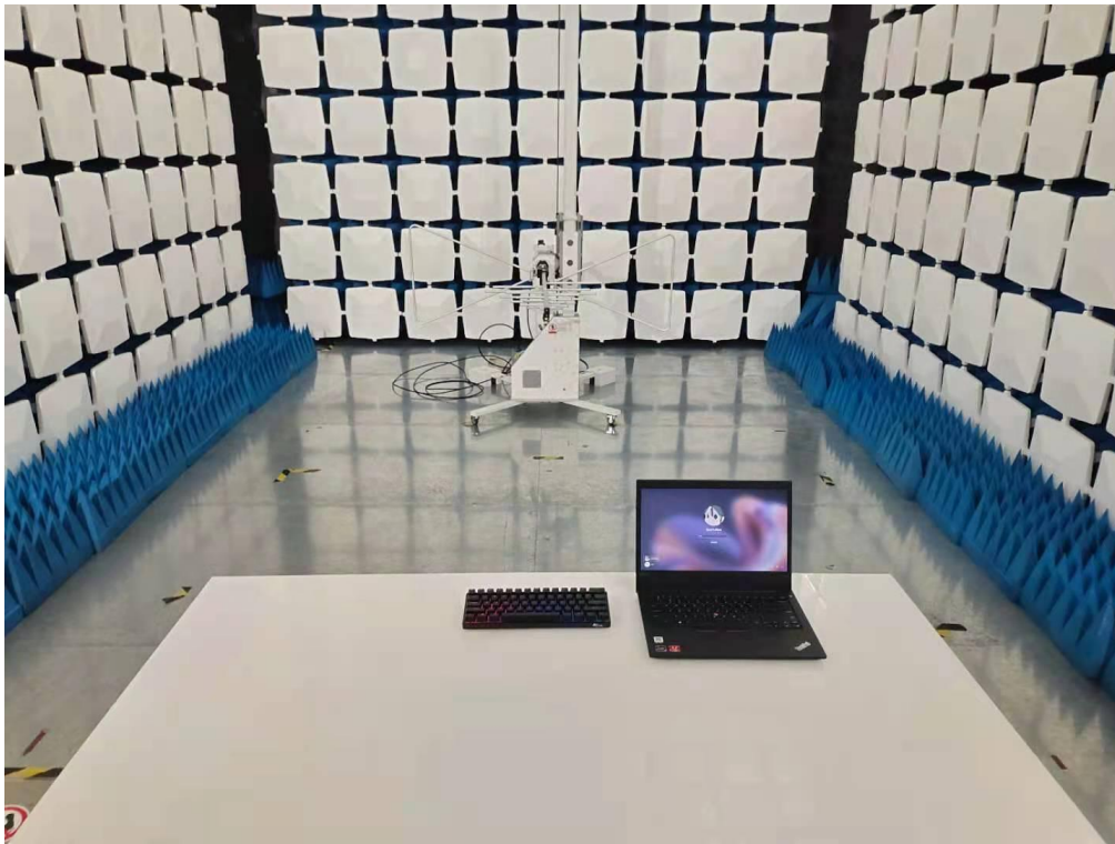
Above 1GHz for radiated emission test setup
