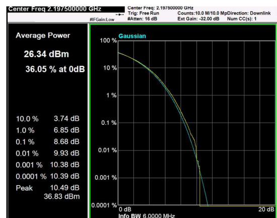
Channel: TOP, Modulation: 16QAM, BW=5MHz, CCDF
