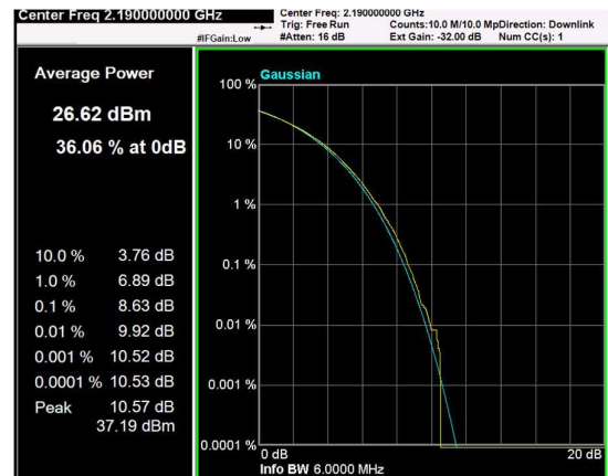
Channel: MIDDLE, Modulation: 16QAM, BW=5MHz, CCDF
