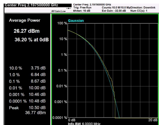
Channel: TOP, Modulation: 256QAM, BW=5MHz, CCDF
