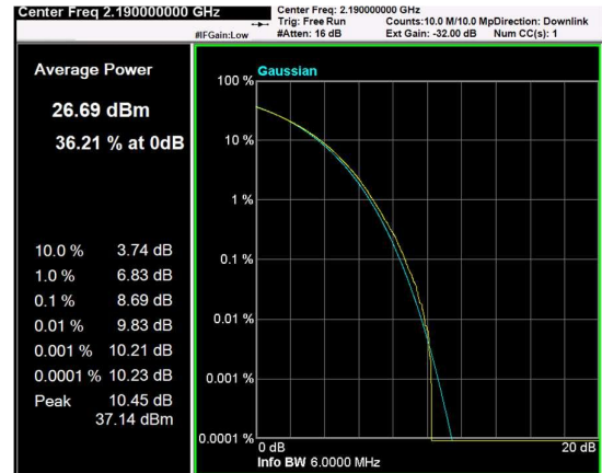
Channel: MIDDLE, Modulation: QPSK, BW=5MHz, CCDF
