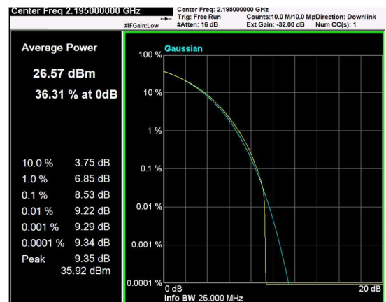
Channel: TOP, Modulation: 16QAM, BW=10MHz, CCDF
