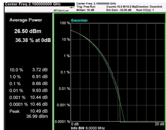
Channel: MIDDLE, Modulation: 256QAM, BW=5MHz, CCDF
