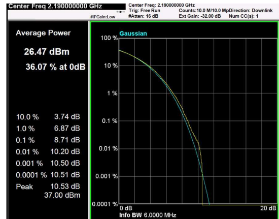
Channel: MIDDLE, Modulation: 64QAM, BW=5MHz, CCDF
