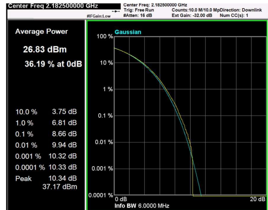
Channel: BOTTOM, Modulation: QPSK, BW=5MHz, CCDF
