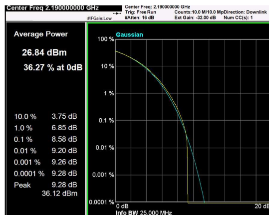
Channel: MIDDLE, Modulation: QPSK, BW=10MHz, CCDF
