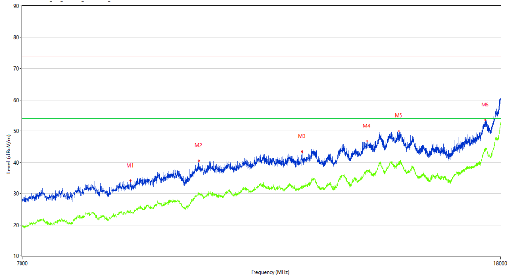
R Emission Test case_FCC_Part 15C_FCC 15.247_7GHz-18GHz
