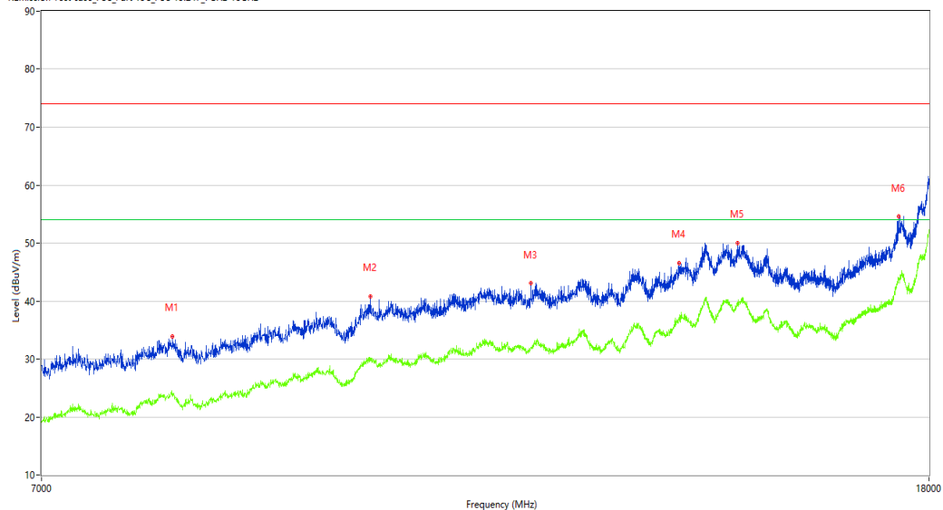
REmission Test case_FCC_Part 15C_FCC 15.247_7GHz-18GHz
