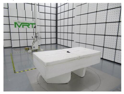
Description: Radiated Emission Test Setup for 1GHz~18GHz
