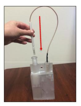
3. Push pin down into the plunger firmly until it clicks into place. Then push the plunger down to arm and lock the sensor.
