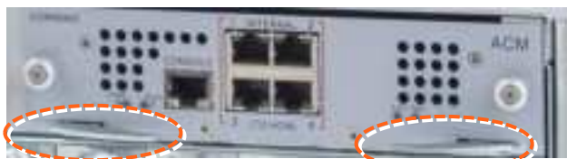
Figure 5: Module Captive Screws and Ejectors
