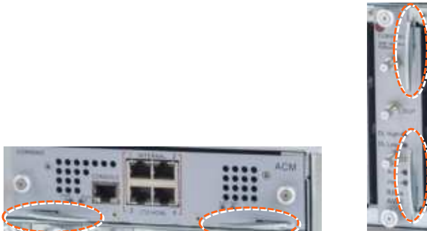
Figure 8: Module Captive Screws and Ejectors
