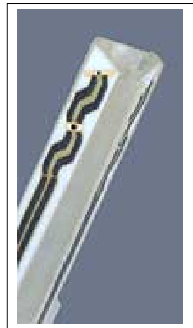
Inside view of ET3DV6 E-field Probe
