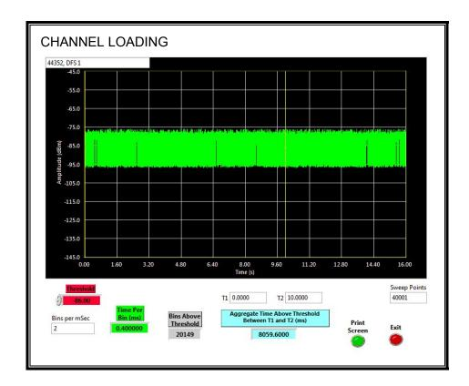
The level of traffic loading on the channel by the EUT is 80.596%.
