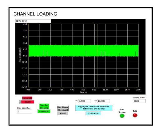
The level of traffic loading on the channel by the EUT is 55.8%.
