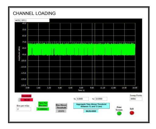
The level of traffic loading on the channel by the EUT is 86.284%.
