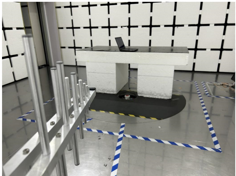
Radiation Emission Test Setup (30MHz to 1GHz)
