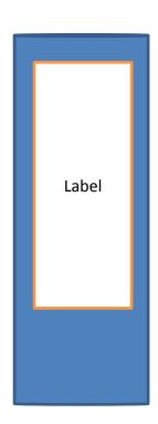
Label is located in the battery compartment under the battery; the customer will see the label when they put the battery in the device.
