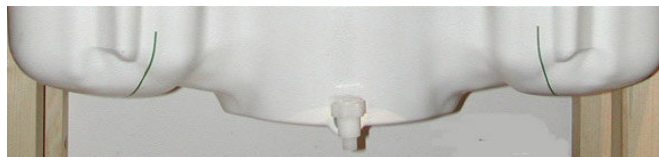
Figure 7.2 SAM Twin Phantom shell
