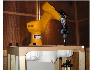
Figure 6.1 DASY4 Test System
