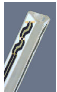
Figure 3.2 Probe Thick-Film Technique
