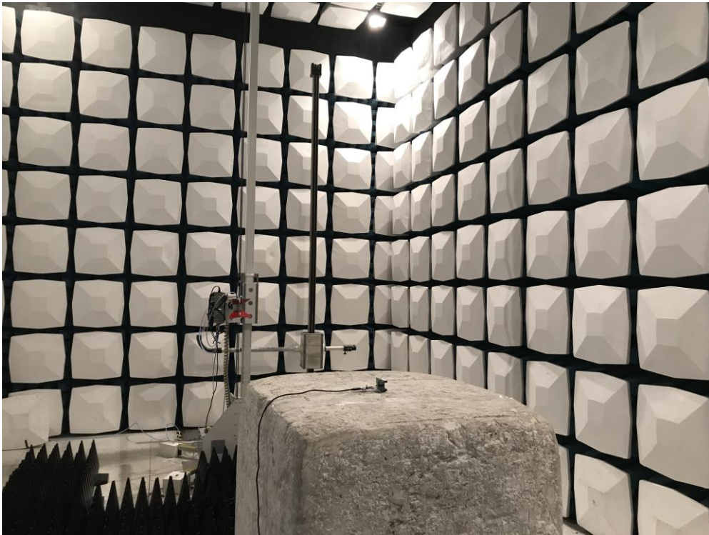
Description: Radiated Emission Test Setup for 1~18GHz
