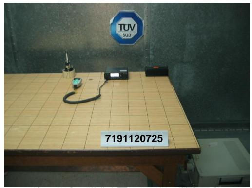
Conducted Emissions Test Setup (Front View)
