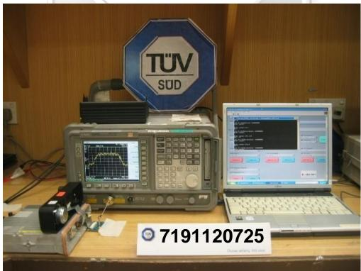
Spectrum Bandwidth (20dB Bandwidth Measurement) Test Setup
