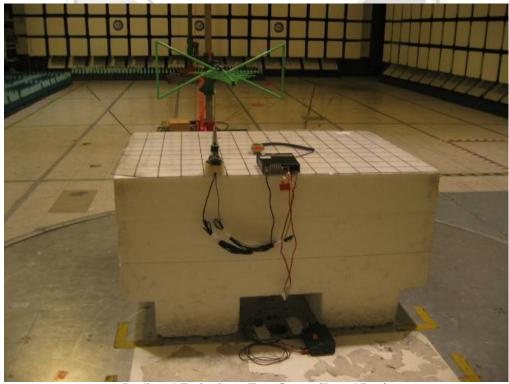
Radiated Emissions Test Setup (Rear View)
