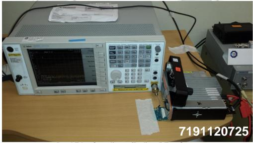
Band Edge Compliance (Radiated) Test Setup
