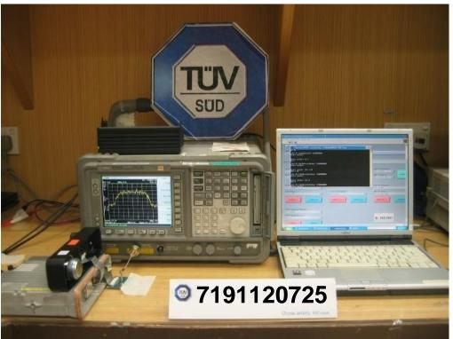
**Carrier Frequency Separation Test Setup**
