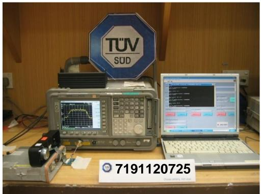
**Peak Power Spectral Density Test Setup**
