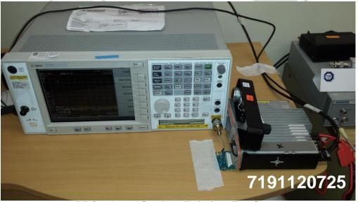
**RF Conducted Spurious Emissions Test Setup**
