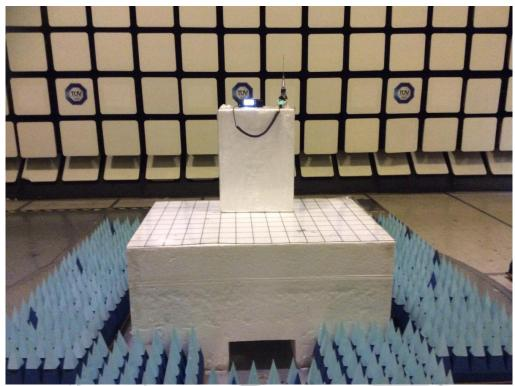
Radiated Emissions Test Setup (Front View)
