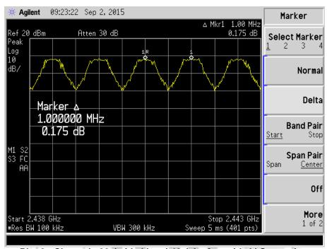
Plot 3 - Channels 39 (mid ch) and 40 (ch after mid ch) Separation
