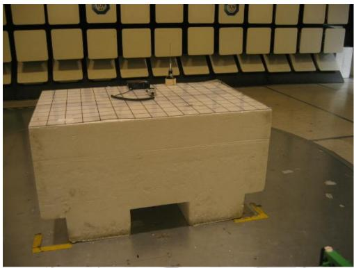
Radiated Emissions Test Setup (Front View)
