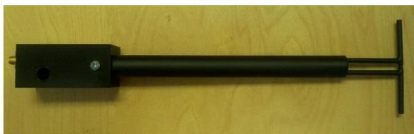
Figure 1 – MVG COMOSAR Validation Dipole
