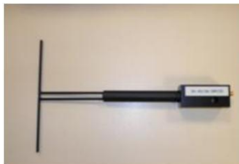
Figure 1 – Satimo COMOSAR Validation Dipole
