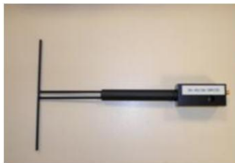
Figure 1 – Satimo COMOSAR Validation Dipole
