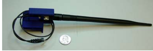
Figure 2.1 External Antenna for Receiving Only
