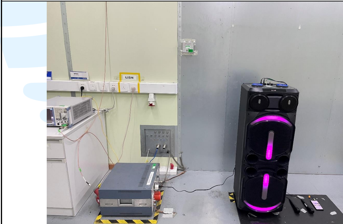
AC Power Line Conducted Emission Test Setup
