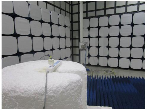
**1.3** Radiated Spurious Emissions Test Setup
