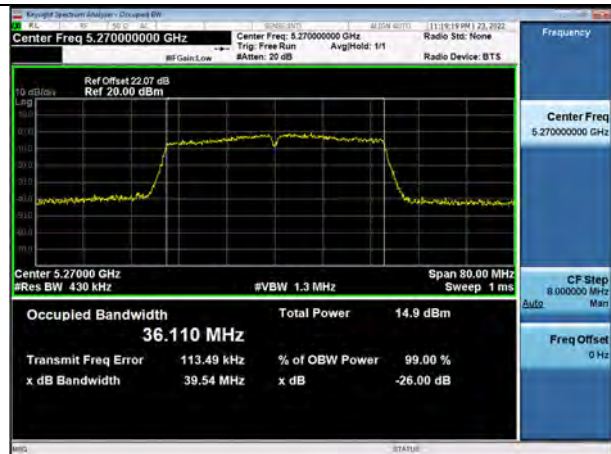
802.11ac_VHT40 UNII 3 BAND 26 dB Bandwidth (CH 151)
