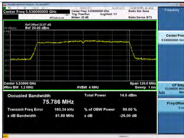
802.11ac_VHT80 UNII 2C BAND 26 dB Bandwidth(CH 106)
