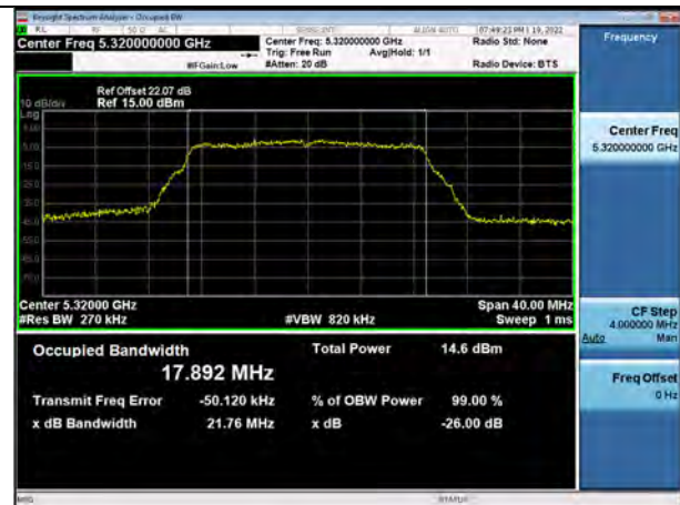
802.11ac_VHT20 UNII 3 BAND 26 dB Bandwidth(CH 157)
