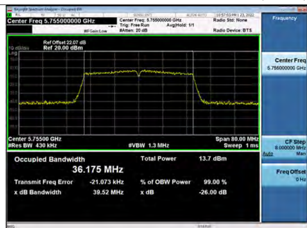
802.11n_HT40 UNII 3 BAND 26 dB Bandwidth (CH 151)
