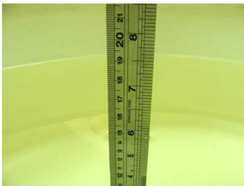
Fig 6.1 Photo of Liquid Height for Body SAR
