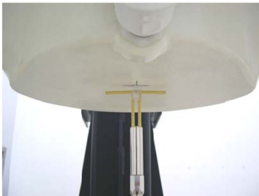
Fig 7.2 Photo of Dipole Setup
