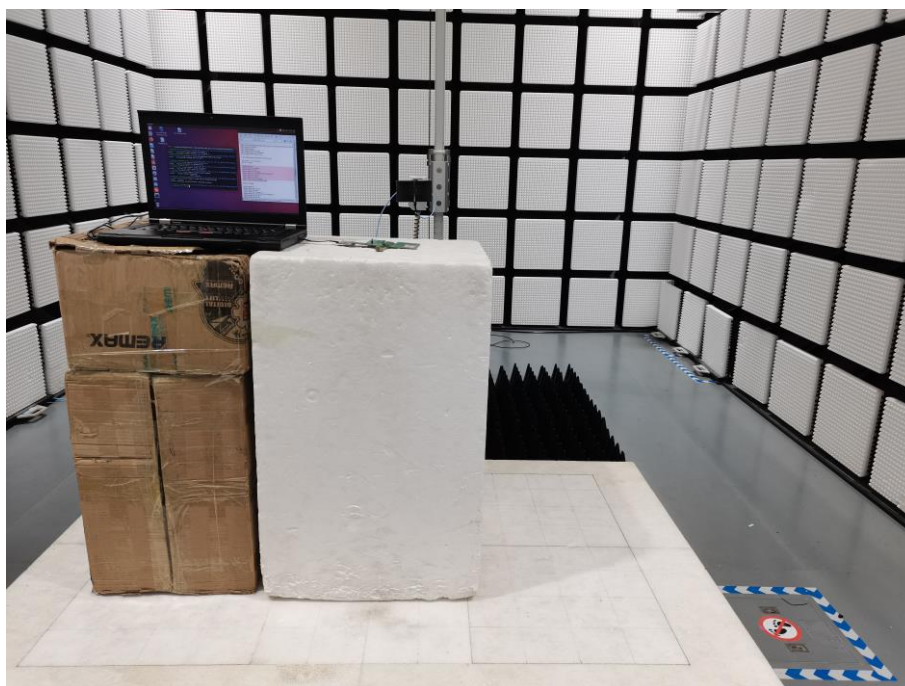
Fig. 3 Radiated emission setup photo(Above 1GHz)
