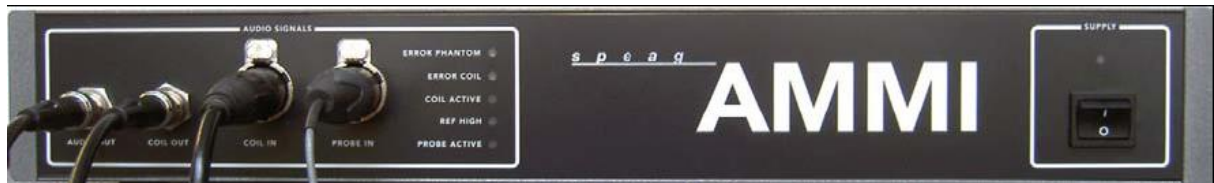
Figure 5.3 AMMI front panel
