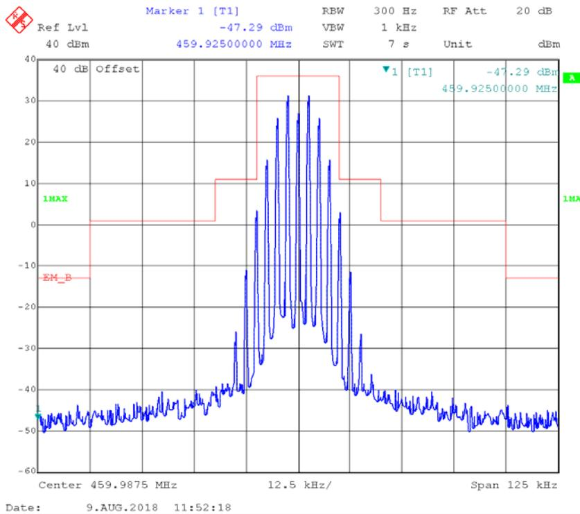
**FM,25kHz,Low Power - Frequency 459.9875 MHz MHz: 99% Occupied & 26 dB Bandwidth**
