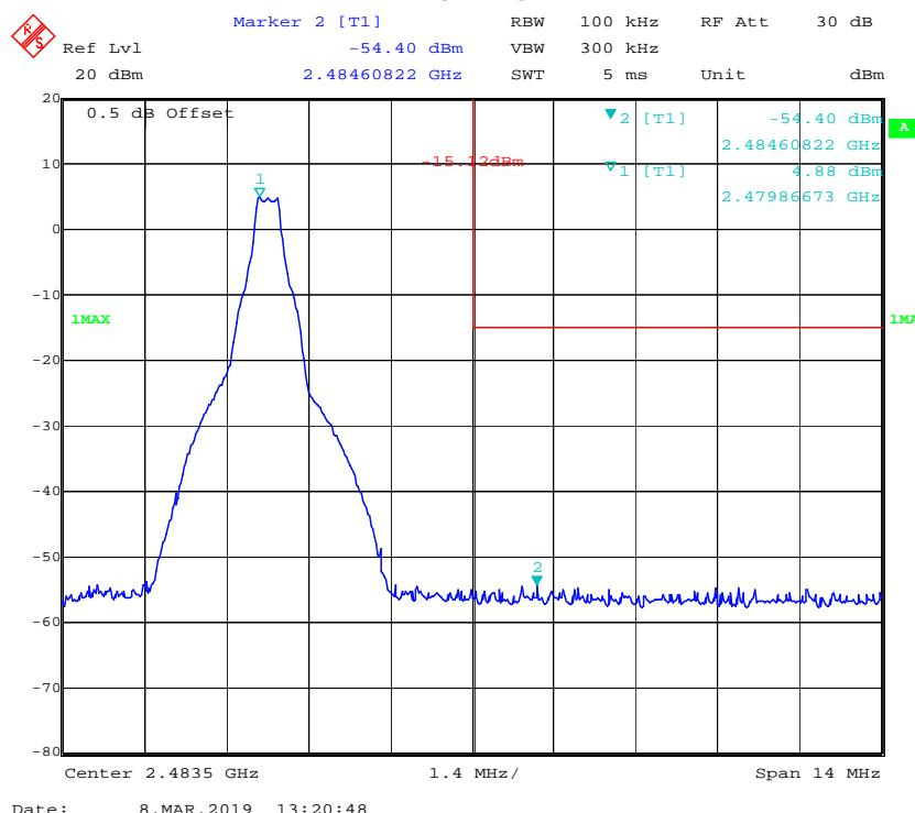
*EDR Mode ( $\pi/4$ -DQPSK):***Band Edge, Left Side**
