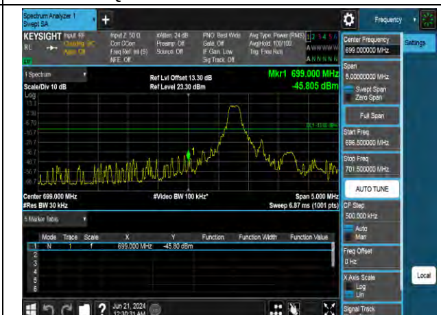
16QAM Low channel-1 RB offset 0
