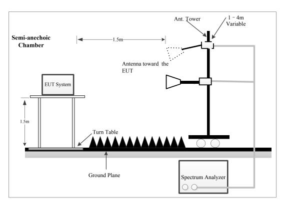
The radiated emission tests were performed in the semi-anechoic chamber, using the setup accordance with the ANSI C63.10-2020. The specification used was FCC 15.209, FCC 15.407 limits.
