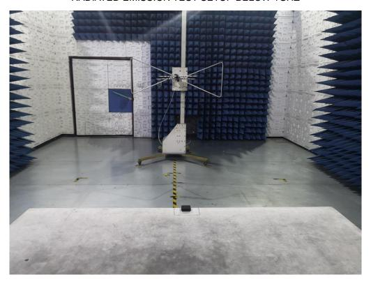
RADIATED EMISSION TEST SETUP ABOVE 1GHZ
