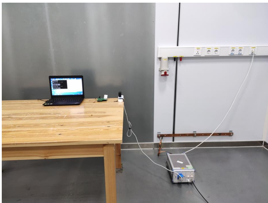
Fig. 4 Power line conducted emission setup photo
