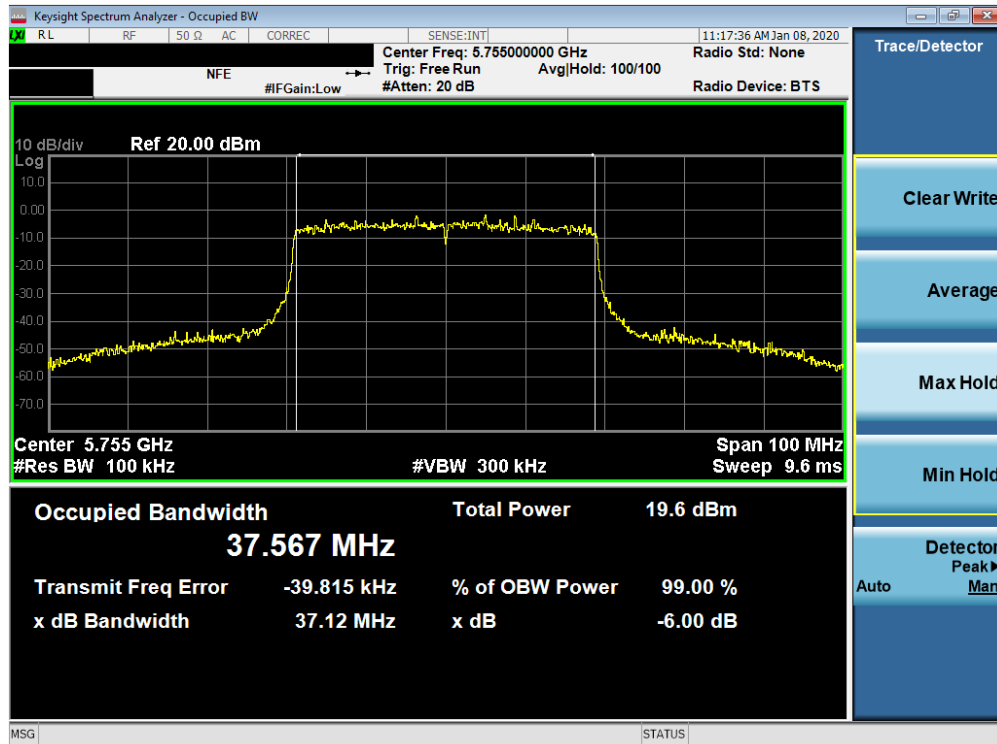
Plot 7-125. 6dB Bandwidth Plot SISO ANT2 (40MHz BW 802.11ax (UNII Band 3) – Ch. 151)
