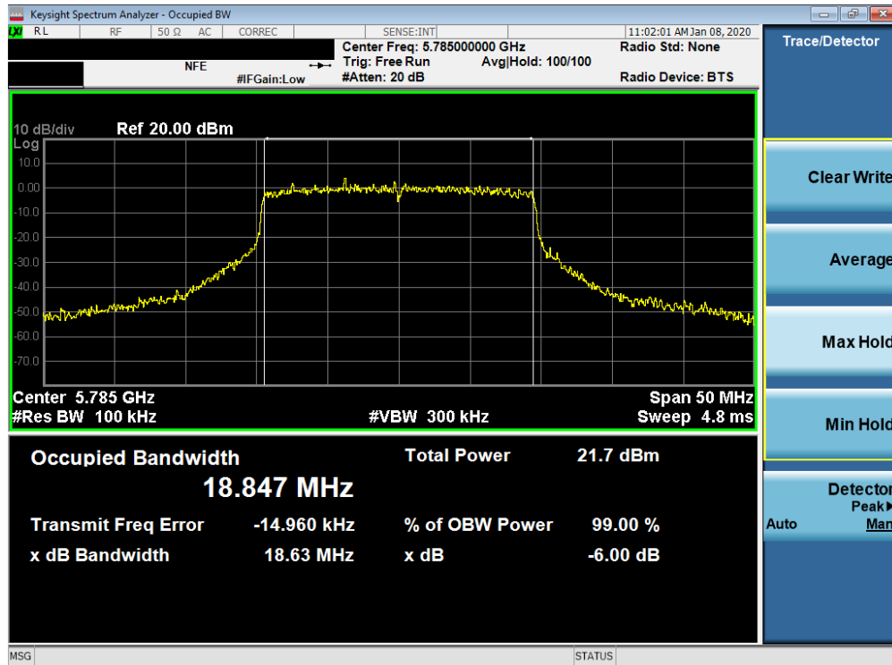
Plot 7-121. 6dB Bandwidth Plot SISO ANT2 (20MHz BW 802.11ax (UNII Band 3) – Ch. 157)
