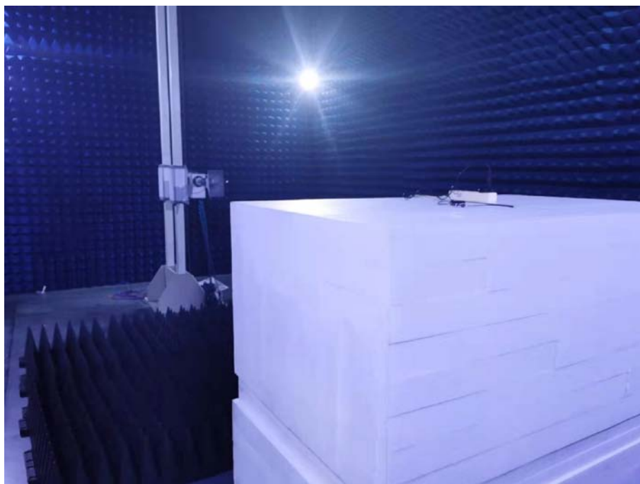
Photo of Radiated Emission Measurement Above 1GHz
