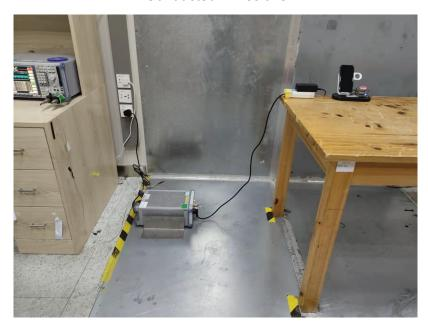
Radiated Emissions From 9kHz-30MHz
