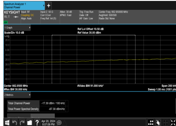
N71(10M)_CP- OFDM_QPSK_Edge_1RB_Left_Low_CH_chp_ PASS
