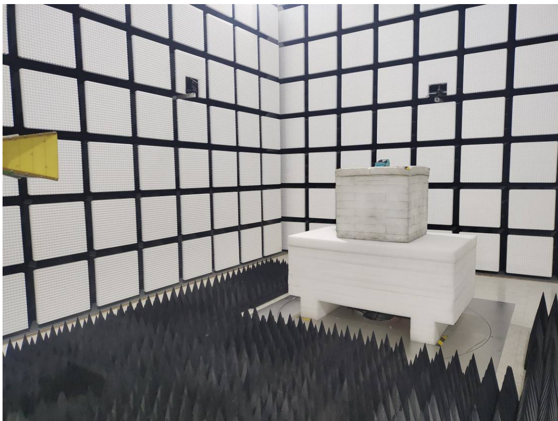
Radiated Emission Above 1GHz View
