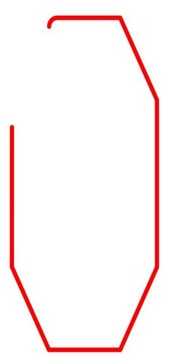
Remote control antenna specification Antenna size: 433.927MHZ, antenna, material: Copper The antenna is whip with a width of 0.8mm a thickness of 1 oz and a total straightening length of 120mm Antenna Gain: OdBi
