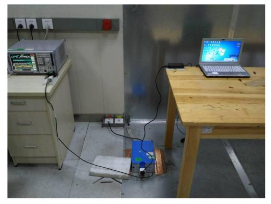
FCC RADIATED EMISSION TEST SETUP
