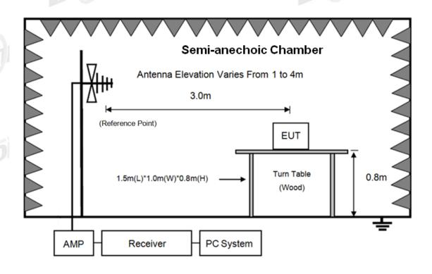
Semi-Anechoic 3m Chamber
