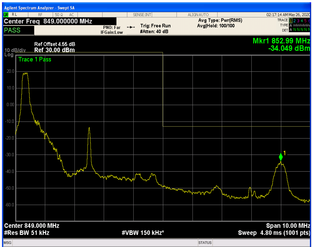
LTE Band5 QAM16 BW=5MHz Channel=20625 RB Size=1 Position=#Max
