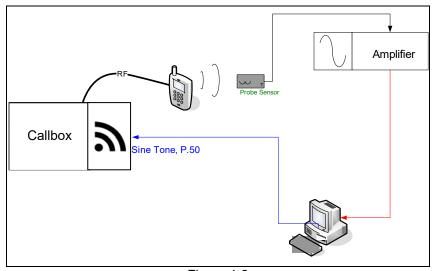
Figure 4-2 T-Coil Test Setup
