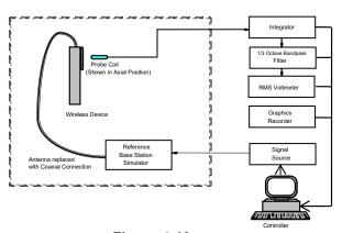
Figure 4-13 **Audio Magnetic Field Test Setup**
