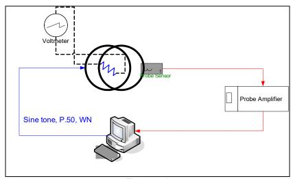
Figure 4-1 Validation Setup with Helmholtz Coil
