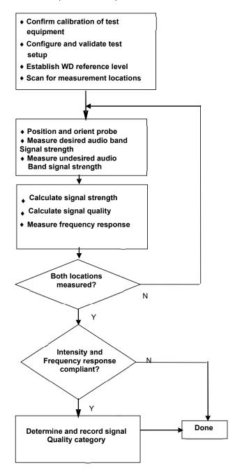
Figure 4-14 C63.19 T-Coil Signal Test Process
