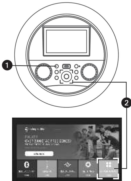
1 Connect the unit as described previously. Press the **⏻ (ON/STANDBY)** button to turn the unit on. The function indicator will light up.
