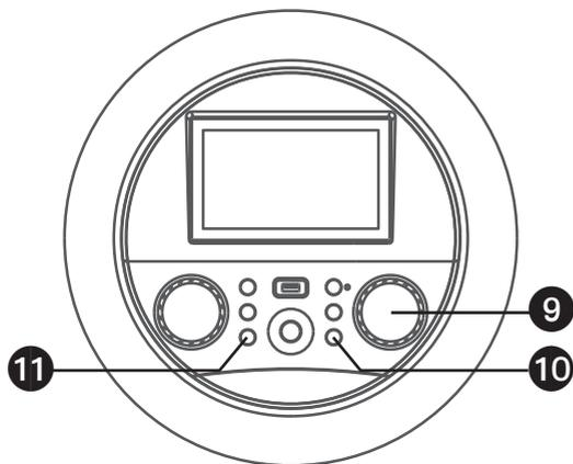
9 Adjust the **MIC VOLUME/ECHO** control as desired. Increasing this control will increase the volume of both microphones. Press then rotate the **MIC VOLUME/ECHO** control as desired to add an echo effect to your voice. Rotate towards **MAX** to increase the echo.
