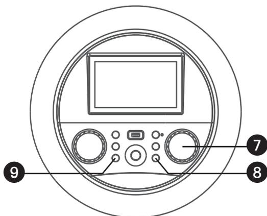
7 Adjust the **MIC VOLUME/ECHO** control as desired. Increasing this control will increase the volume of both microphones. Press then rotate the **MIC VOLUME/ECHO** control as desired to add an echo effect to your voice. Rotate towards **MAX** to increase the echo.
