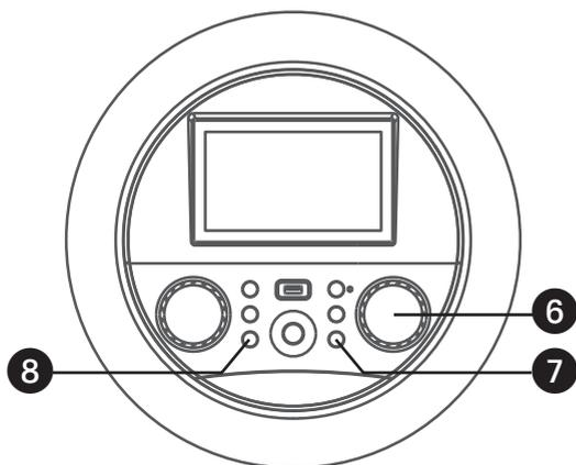
6 Adjust the **MIC VOLUME/ECHO** control as desired. Increasing this control will increase the volume of both microphones. Press then rotate the **MIC VOLUME/ECHO** control as desired to add an echo effect to your voice. Rotate towards MAX to increase the echo.
