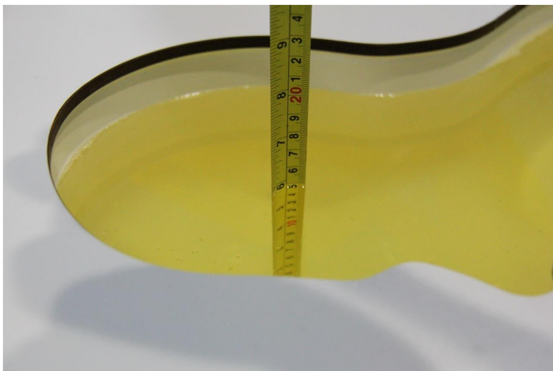
Picture 7-2 Liquid depth in the Head Phantom (2450MHz)
