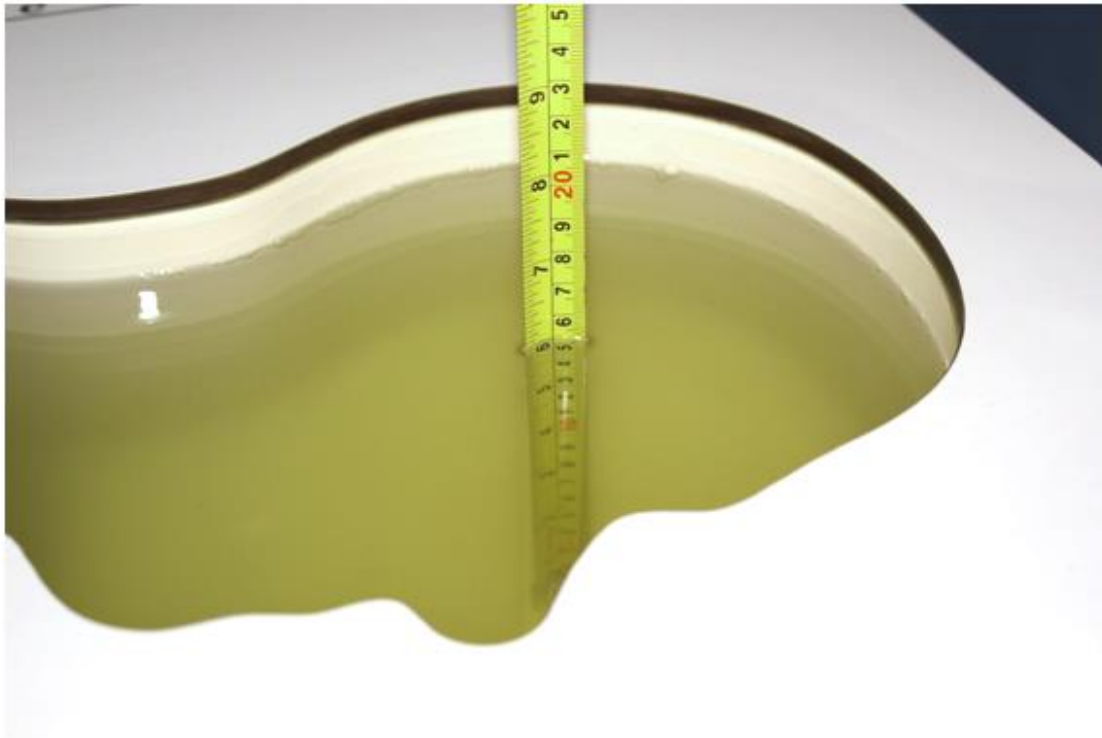
Picture 7-3 Liquid depth in the Head Phantom (2600 MHz)
