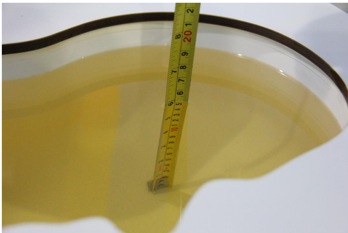
Picture 7-1 Liquid depth in the Head Phantom (900 MHz)
