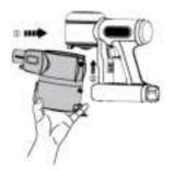
When re-attaching the dustbin, hold on an angle and slot the top of the dustbin into the hook on the main body. Push upwards until the hook is fixed into the slot on the dustbin and then it clicks back into place.
