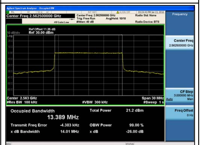
LTE band 7 - Middle CH 16QAM-15
