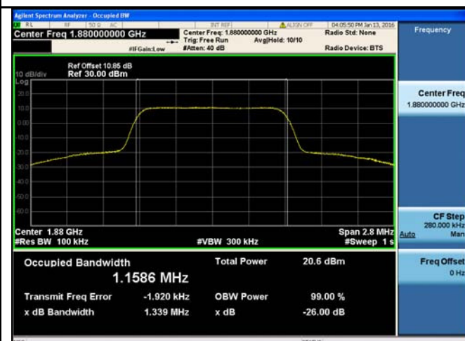
LTE band 2 - Low CH 16QAM-1.4
