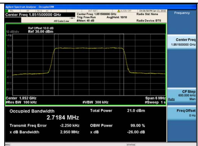
LTE band 2 - Low CH 16QAM-3
