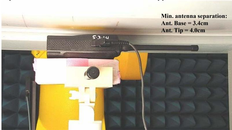
Figure 13: Robot Test System (Flat Phantom)
