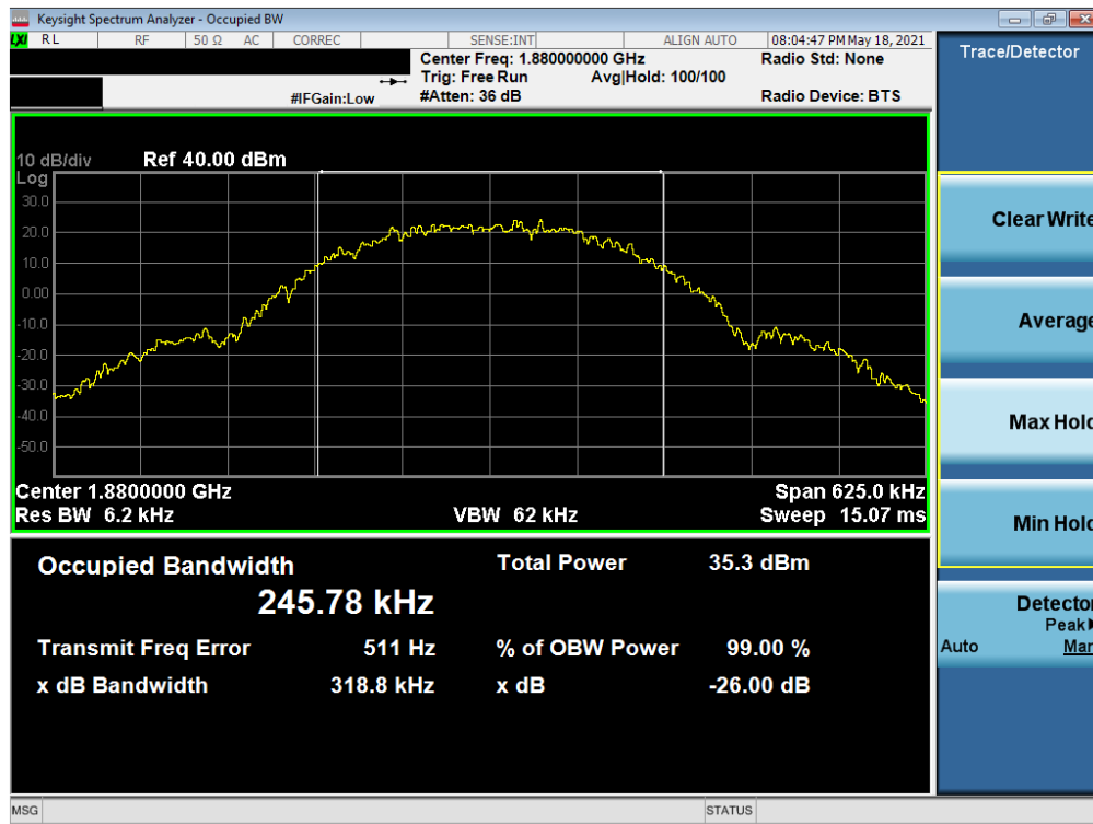
Plot 7-13. Occupied Bandwidth Plot (GPRS, Ch. 661)
