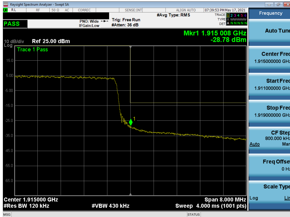
Plot 7-59. Upper Band Edge Plot (LTE Band 25 - 10MHz QPSK – Full RB)
