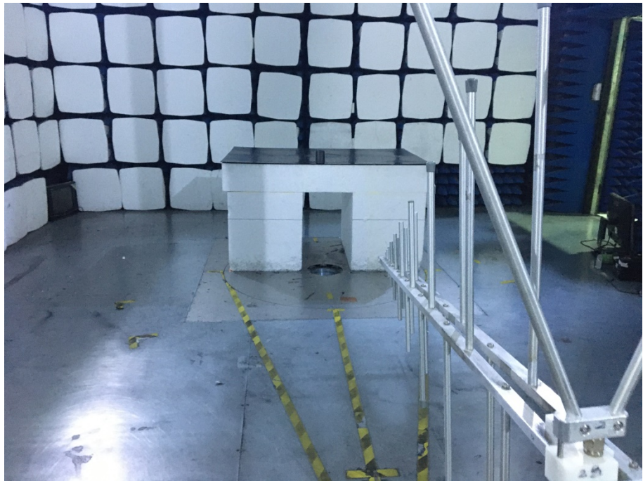
Radiation Emission Test Setup (30MHz to 1GHz)
