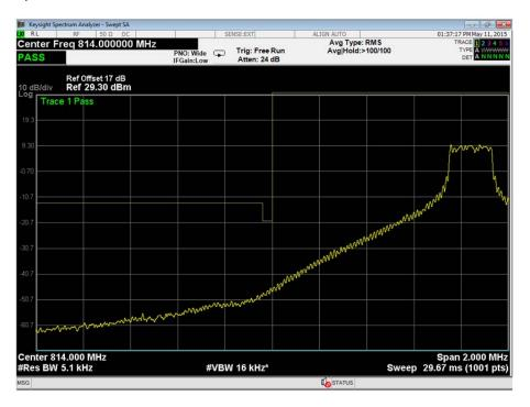
LTE FDD 26, 821.5 MHz, All Resource Blocks, 15.0 MHz Bandwidth, QPSK, Block Edge, Spurious at Antenna Terminals Results
