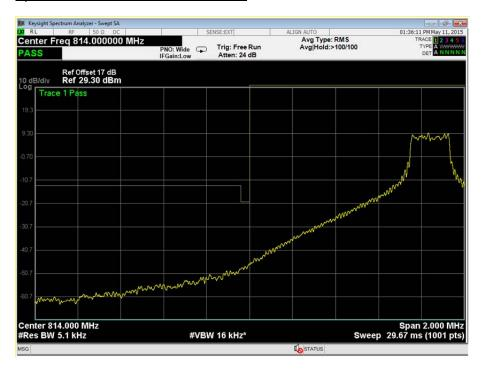
LTE FDD 26, 821.5 MHz, All Resource Blocks, 15.0 MHz Bandwidth, 16-QAM, Block Edge, Spurious at Antenna Terminals Results
