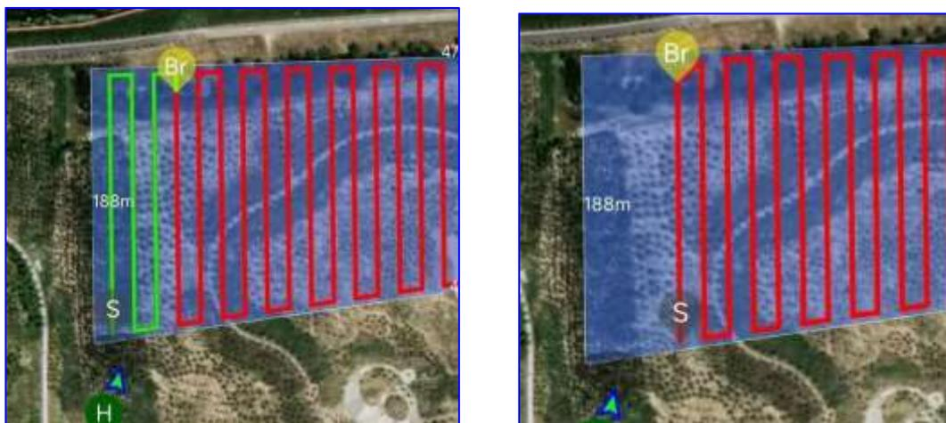
**Move Navi.:** adjust the overall deviation of the plot. You can use the Move Navi. function to move the entire flight route.
